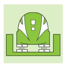
Let us study how the train levitates. There are permanent magnets on the bottom of the train, and electromagnets on the tracks. By providing power to the electromagnets, they generate a magnetic field, thus repelling the permanent magnets and applying an upwards force on the train. Because the magnetic field is stronger at shorter distances, for the same amount of power, the repulsion is stronger when the train is lower, and weaker when the train is higher.
